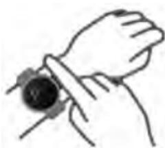
The smartwatch should rest at a finger's width below your wrist bone. The bottom of the smartwatch should be slightly in contact with your skin. Keep the smartwatch secured on wrist during workouts.
