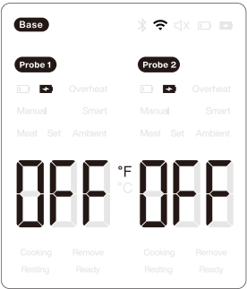
Probe charging and Base Not Charging
