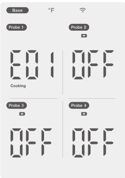
Probe Malfunction, Error Code EXX Reported
